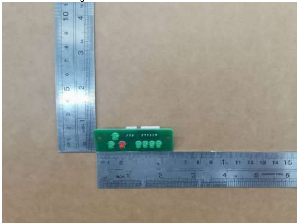
Figure 9. The led PCB for models AM-10
