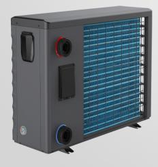
Inverboost technology is an air to water heat pump to heat & cool the water of a pool / jacuzzi. It includes Full Inverter technology to automatically adapt the compressor and fan speed to the heating needs and weather conditions. The Mitsubishi compressor, pcb and fan motor adopt the inverter technology. The result is a very quiet and low energy consumption heat pump. The units work silently in both silent or smart mode. To ensure proper efficiency always use a bigger pump than required.
